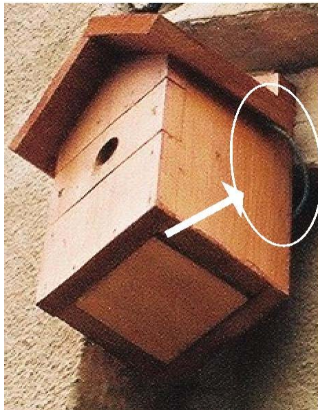
Birdcam in situ - note the cable coming out from under the roof and going round the back where it goes into the house through a hole in the wall
